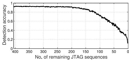
Fig. 7. Detection accuracy is evaluated iteratively, and in each iteration, the sequence with the least impact on the detection accuracy is discarded.
